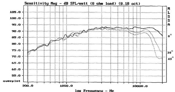
Measured on IEC baffle using Bruel & Kjaer 3144 model microphone. Also available in black faceplate finish.
