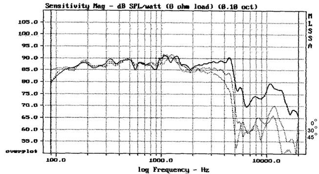
Measured on IEC baffle using Bruel & Kjaer 3144 model microphone.
